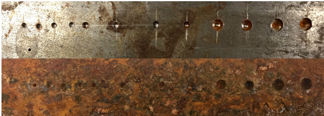
Figure 1: The top picture is the initial carb on steel plate and the one below is the same part at the end of the galvanic corrosion test.
