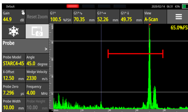
Images above show toe crack on A-Scan and Ray Tracer
