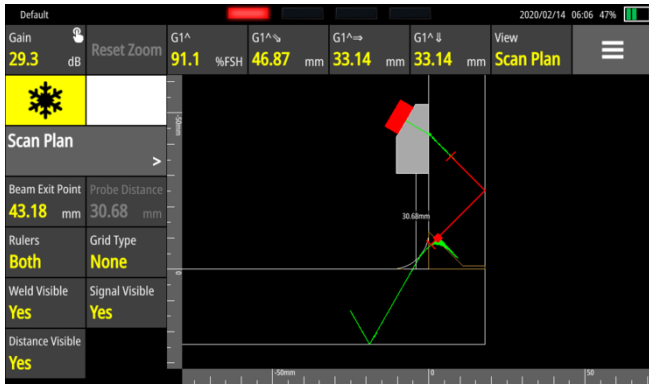
Images above show lack of side wall fusion on A-Scan and Ray Tracer
