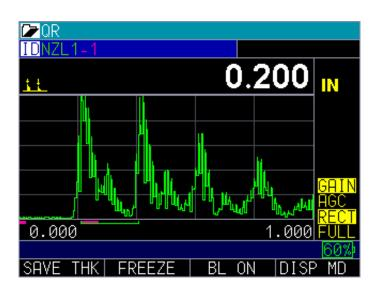
ECHO To ECHO on, see top left yellow peak symbol, also main bang and blank after first detected are on, see fushia colored lines on the bottom of the screen.
