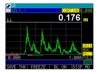
After a two-point substrate thickness and coating velocity cal, we display both substrate and coating thickness.
